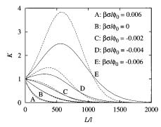
**Figure 6.** Partition coefficient for various values of  $\beta \sigma l \phi_0$  with  $\kappa R = 0$  (dashed) and with  $\kappa R = 1.0$  (solid) from the perturbation theory.
