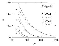
**Figure 8.** Partition coefficient with a strongly repulsive pore wall  $(\beta \sigma l \phi_0 = 0.01)$ , calculated from variational theory (solid) and perturbation theory (dashed).
