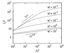
**Figure 4.** Effective step-length  $I_e$  as a function of chain contour length L for different values of  $\kappa l$ . (w/l=1, and  $w_cl=0.1$ )
