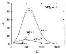
**Figure 9.** Partition coefficient with a strongly attractive pore wall  $(\beta\sigma l\phi_0=-0.01)$ , calculated from variational theory (solid) and perturbation theory (dashed).
