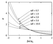
**Figure 3.** Partition coefficient K of a polyelectrolyte in the small radius of gyration limit. K is identical to the partition coefficient of a colloidal particle with charge  $\sigma L$ .
