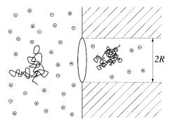
Figure 1. Schematic view of a polyelectrolyte partitioning into a cylindrical pore. The pore wall is maintained with fixed electrostatic potential, and the ions are floating around.
