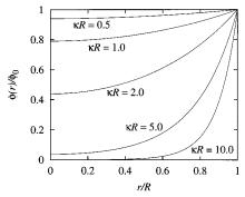
**Figure 2.** Electrostatic potential inside the cylindrical pore for various values of  $\kappa R$ .
